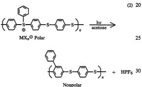
More importantly, one of the intermediates involved in the photo-decomposition process shown in Equation <sup>35</sup> 2, has the same electronic structure as does the known conducting polymer derived from the doping of PPS with powerful oxidizing agents (Scheme I). Thus, the photolyzed regions of our polymer is converted from an insulator to a conductor if ways of "trapping-out" this 40 electronic structure could be devised.
