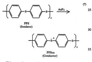
This one electron oxidized form, PPSox, is the same species which is generates by the removal of a phenyl  $_{40}$ radical upon photolysis of our sulfonium PPPS materials (Equation 8).
