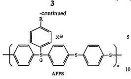
Based on the known chemistry of triaryl sulfonium salts, upon photolysis, these materials undergo a photochemical rearrangement which result in a change in 15 niques, these APPS materials become our "paper" in their character from polar (ionic) to nonpolar and hence allow them to act as a photoresist materials (Equation 2).
