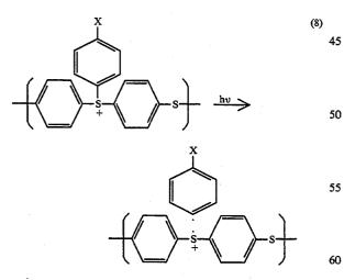
Our approach is to conduct the photolysis of our PPPS derivatives under conditions in which we can quench the reaction following the initial homolytic cleavage which liberates the phenyl radical shown in 65 chemical modification upon reaction with excess AsF5 Equation 8. Doing so gives us the same material as that generated by the oxidation of the parent PPS (Equation 7). In order to inhibit any of the subsequent steps in the
