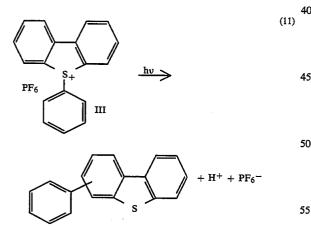
We believe that phenylation of the dibenzylthiophene polymer, Polymer III', is expected to occur on both the thiophene moiety and the sulfide moiety. Preliminary 60 competition experiments that we conducted indicate that both moieties are phenylated under the pertinent reaction conditions. Photolysis of either, both of these sulfonium centers should give a highly conducting material. 65
