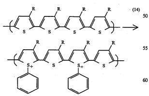
These polythiophene materials offer simplified photochemistry in that no chain scission processes are now 65 possible. Conductivities near  $10^2 \Omega^{-1} \text{cm}^{-1}$  can be obtained upon doping polythiophenes. Utilization of the same basic sulfonium ion photochemistry outline above
